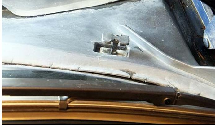
**2)** Lift up cowl corners and inspect for debris. Clear debris.
