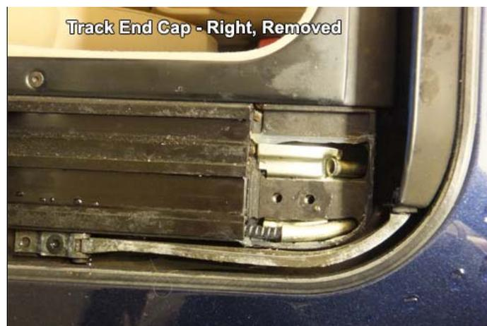
2) After cleaning, apply a bead of silicone caulk to both mating surfaces and reinstall end cap. Apply additional silicone to inside edge and between track gap and end cap. In other words, caulk all sides of end cap generously.
