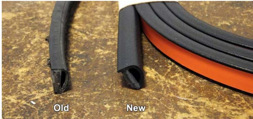
**1)** Remove old seal beginning at rear center seam. Grab and pull strongly to separate seal adhesive from roof opening.
