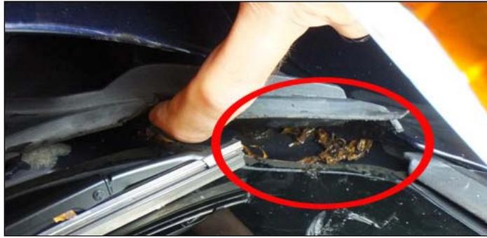
But there's even more. The sunroof's outer seal is the first line of defense against water intrusion. But over time, the seal degrades, allowing much more water to pass. The seal part number has been superseded (updated) by BMW no less than 5 times, indicating this is a known problem. It's likely the sunroof seal on your car hasn't been updated since it left the factory.
