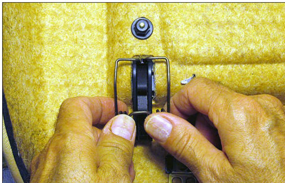
**5) Next, remove the two (2) 10mm black plastic retaining nuts. Repeat for other side:**
