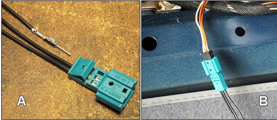
Solder or crimp the loose ends to the wires of the Resler interface using this schema:
