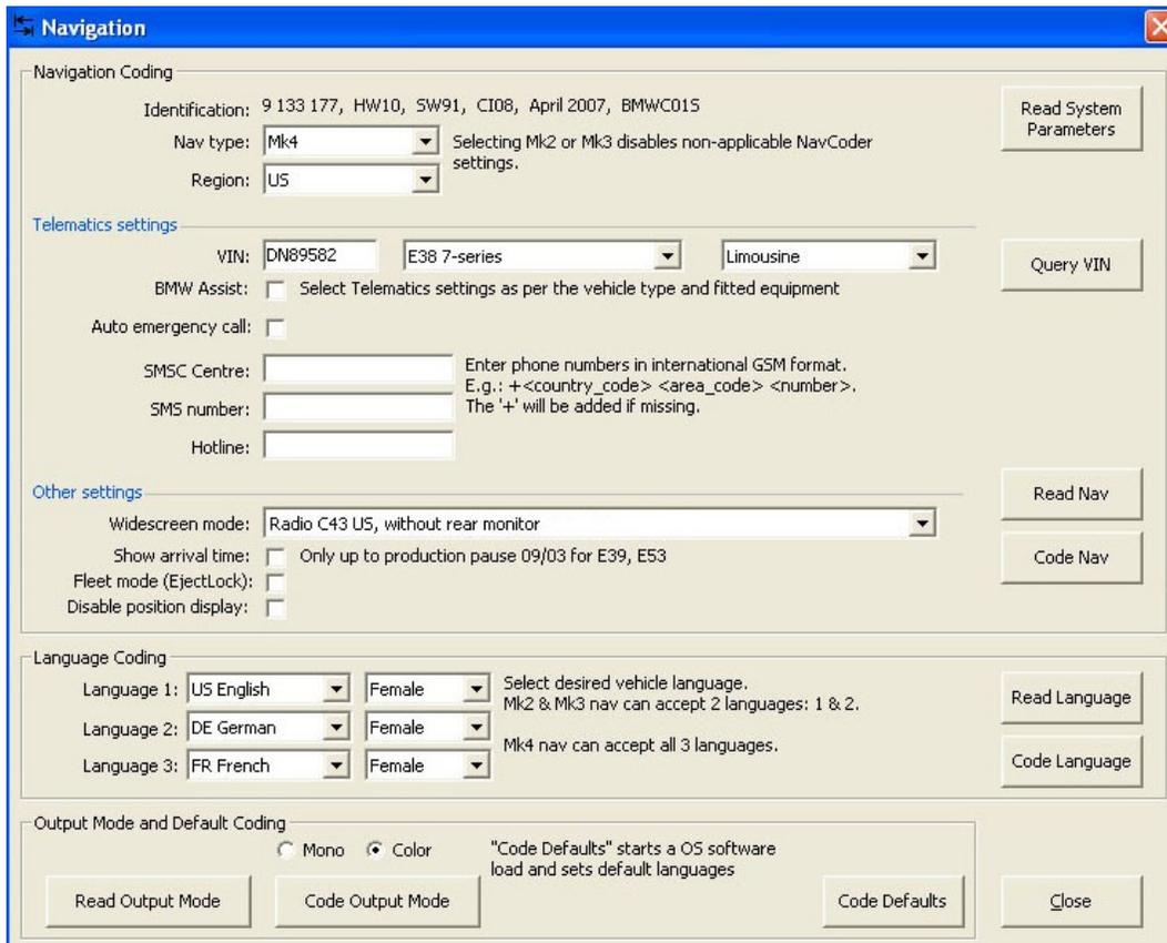
Click the *Read Nav* button (middle right) to get the configuration of the nav computer currently connected (hopefully, your new Mk4!).
