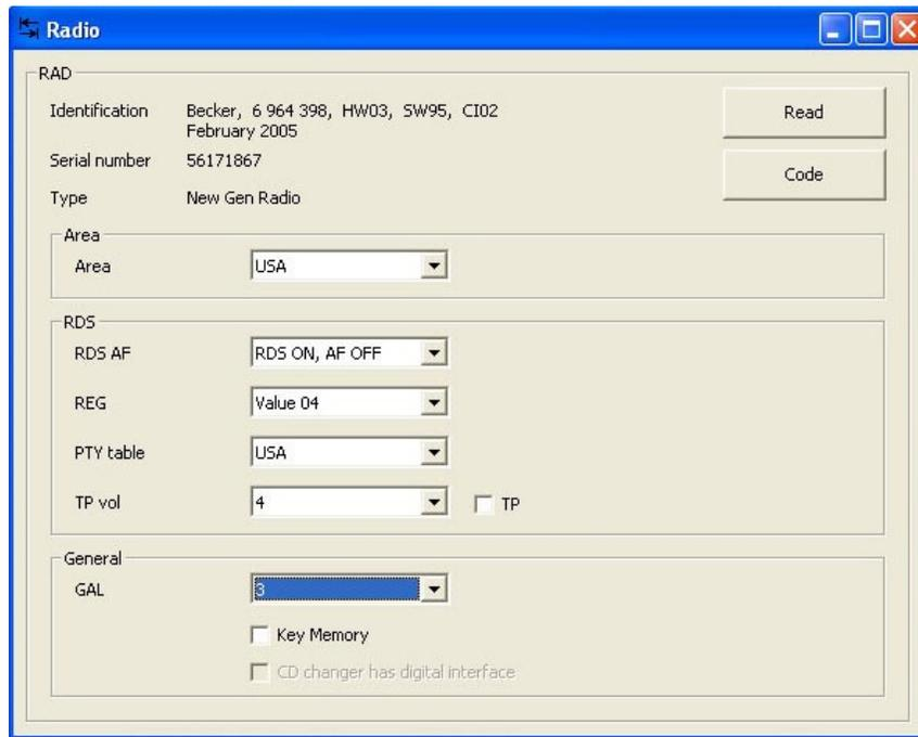
Radio coding is typically not required and is simply a "nice-to-know" feature. However it can be of use when installing new but used radios, such as when upgrading from standard C43 navigation radios to New Gen radios (or CD43/CD53 in-dash radios).
