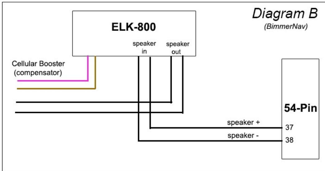
Reference the diagram printed on the amp's label for connections at the ELK-800. Strip 1/4" off the ends of each wire and secure them into the terminals of the amp by turning the small screw atop each respective binding post.
