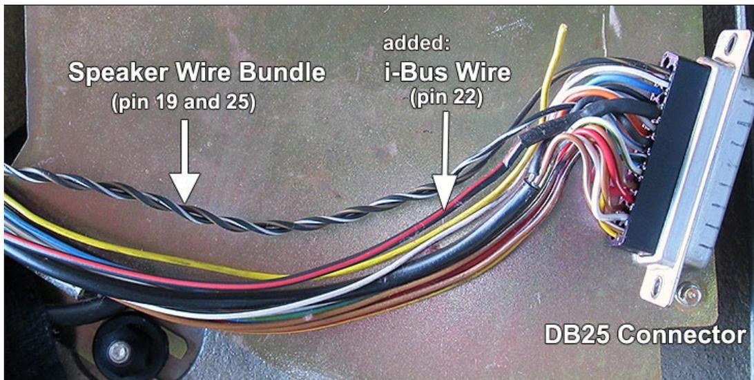
3) With the ELK-800 securely mounted in its location, snip the needed wires of the DB25 bundle in the most convenient place for access to the amp's terminals, according to this schematic:
