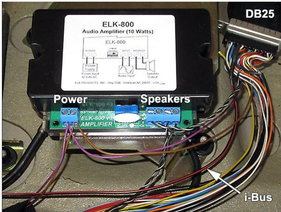
5) Re-wrap the DB25 wire bundle as appropriate and verify both amp and wire bundle are secure. Image below shows an installation in a '99 528iT, with both TCU and ELK-800 secured to mounting boards atop existing factory brackets.
