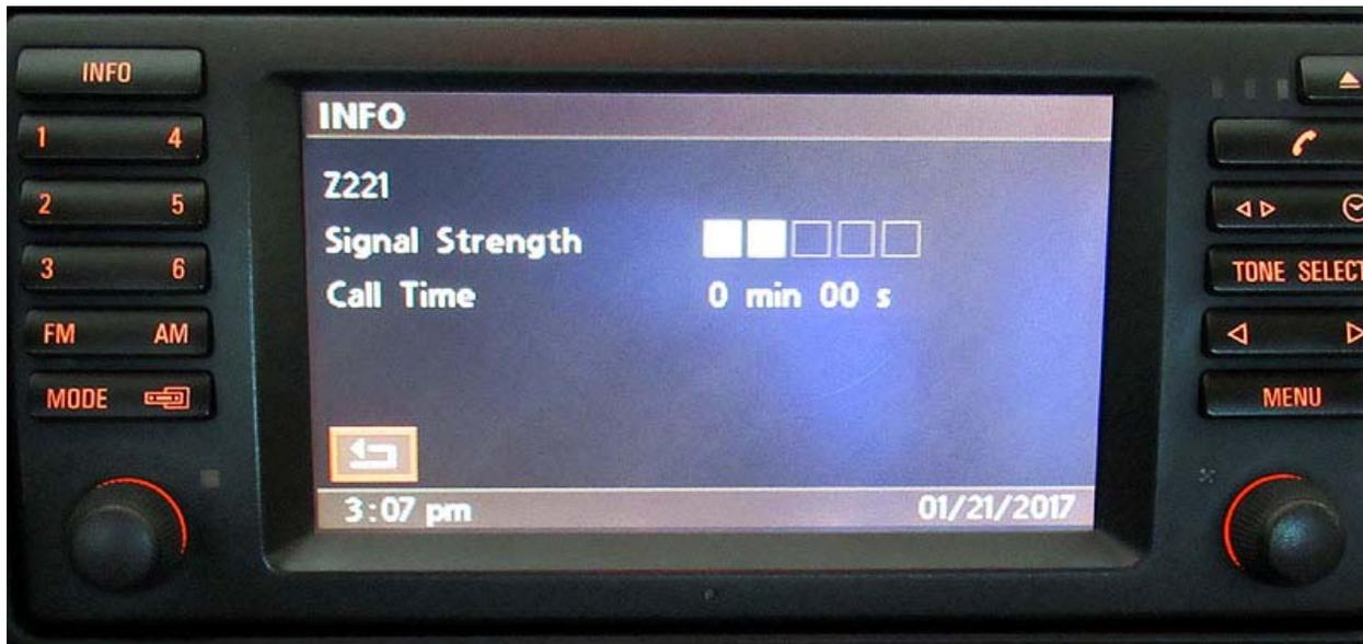
"Signal Strength" represents the phone-to-tower signal, not the local phone-to-antenna signal. I didn't realize this information was available in the Bluetooth protocol. It's cool that BMW includes this feature.
