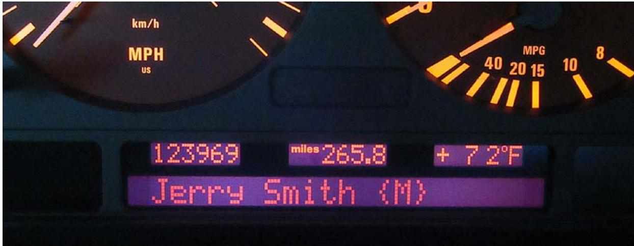
Press the R/T button on steering wheel to bring up Directory in cluster (regardless of radio/screen status). Scroll thru it using Up/Down arrows (hold down to go fast). Press speech button to call, and press again to terminate call.
