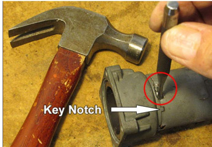
Re-stake using punch tool. NOTE: case parts are keyed for correct installation. Verify alignment of key notch (see image above).
