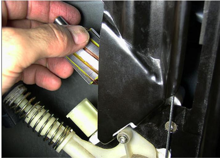
With window closed, the gearbox will be under tension. Hand-turn motor shaft counter-clockwise about 3-4 revolutions to release tension. See image above. When motor shaft feels loose, wiggle and pull it free from gearbox, along with circuit panel.
