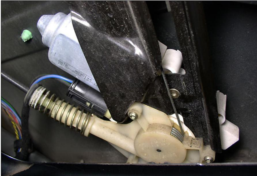
The motor will reside behind the black regulator frame and therefore be partially obscured. The motor's white plastic gearbox is screwed to the cable drive in front, with an attached electric plug. Remember, your car's set-up will vary depending on model year and door. (530i right rear door shown above.)
