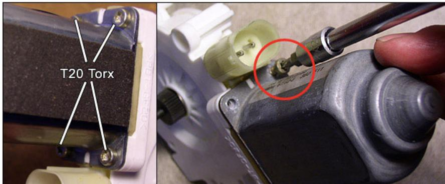
Visibility will be limited. Use an inspection mirror to help locate screws. Magnetize your torx driver to help prevent dropping screws as they're removed. If dropped, use tweezers to extract.
