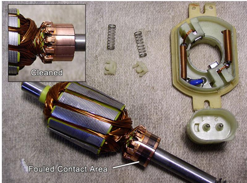
We've finally reached the heart of the problem. Using steel wool or equivalent, clean copper contact area on motor shaft. See image above. Clean also contact points on circuit panel and any other parts that contain dirt or dust. Done!
